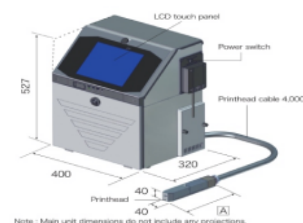
Main Unit /Printhead Dimension
